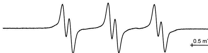
Fig. 10. ESR spectrum of the spin adduct formed upon heating a solution of TME ozonized at -60^{\circ}\text{C} with PBN in heptane at 80^{\circ}\text{C} .
